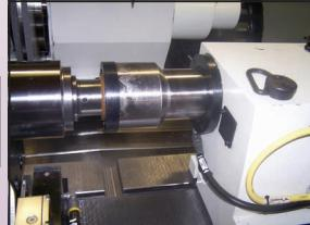
High pressure wheel cleaning and air-knife for part blow-off
