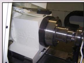
Live spindle work head with hydraulic face driver
